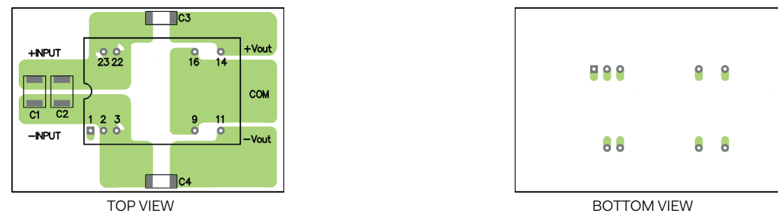
Fig. 4-3 Recommended Layout Pattern for Dual Output
