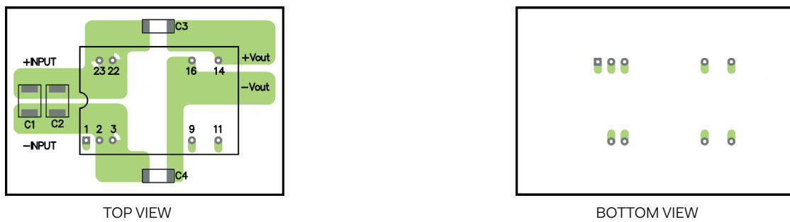
Fig. 4-2 Recommended Layout Pattern for Single Output
