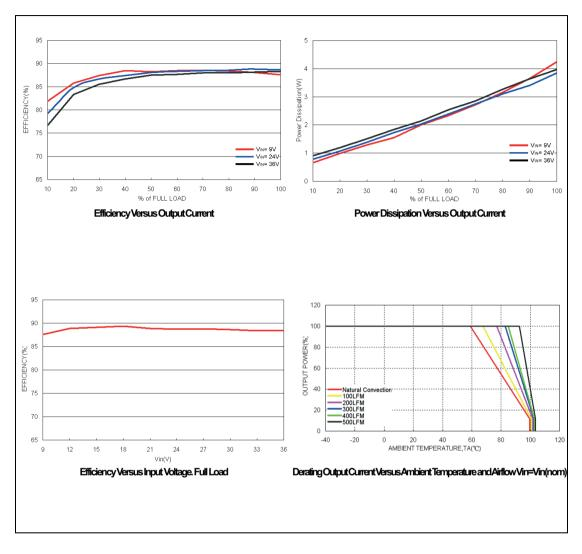
All test conditions are at 25°C.The figures are identical for PMC30-24D15W
