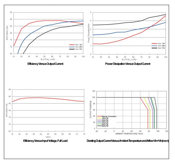
All test conditions are at 25°C.The figures are identical for PMC30-48D05W
