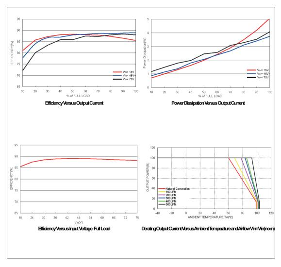
All test conditions are at 25°C.The figures are identical for PMC30-48D15W
