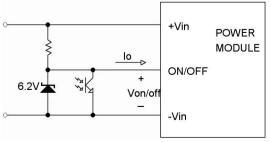
Level Control Using Line Voltage
