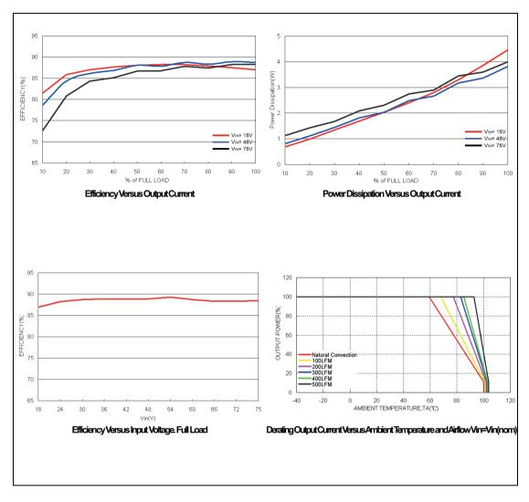
All test conditions are at 25°C.The figures are identical for PMC30-48D12W
