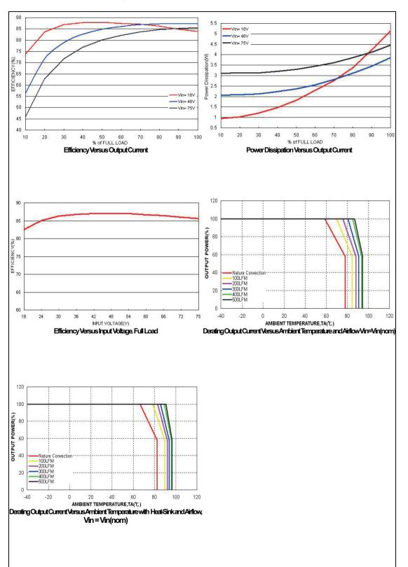
All test conditions are at 25°C.The figures are identical for PMC30-48T3312W
