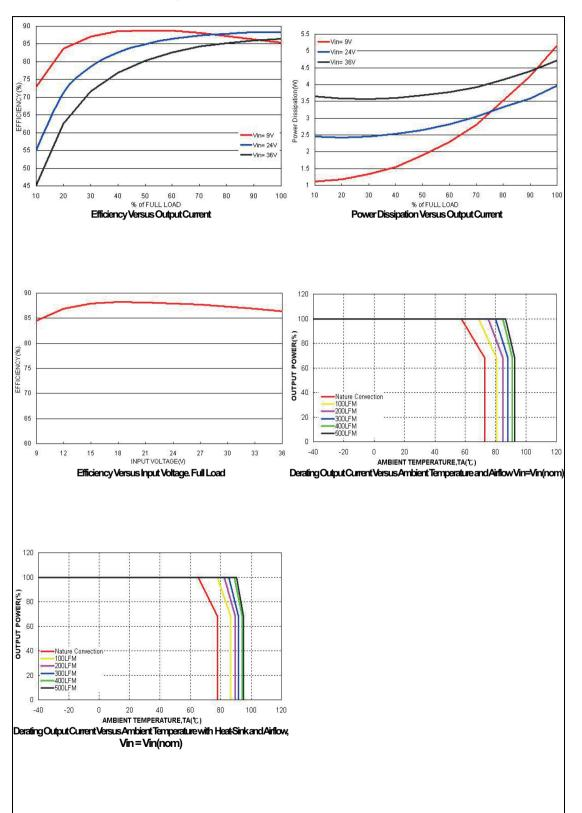
All test conditions are at 25°C.The figures are identical for PMC30-24T0512W
