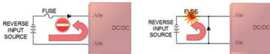
Fig Reverse input voltage protection
