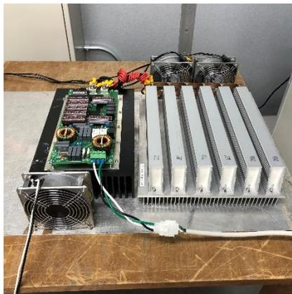
Fig. Conducted emission test environment
