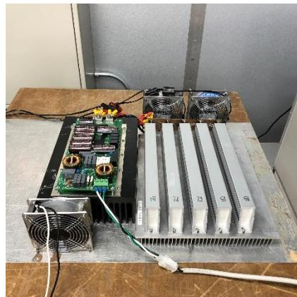
Fig. Conducted emission test environment
