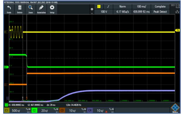
Turn OFF AC input Load Current : 25A
