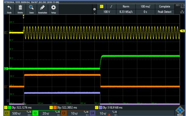
Turn ON AC input Load Current : 25A
