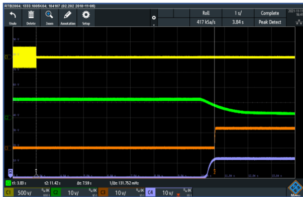
Turn OFF AC input Load Current : 0A (1s/div)
