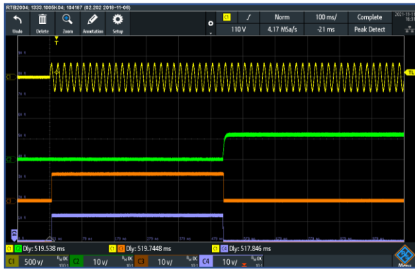
Turn ON AC input Load Current : 0A (100ms/div)
