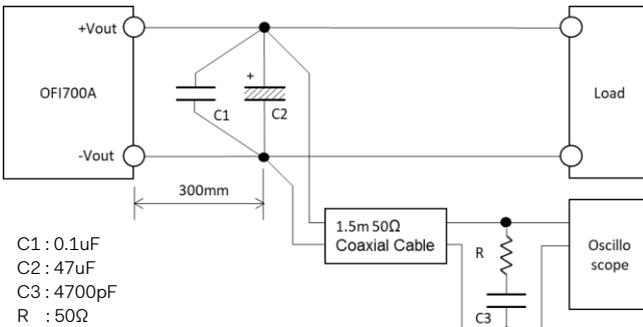
Fig.3.3 Method of Measuring Output ripple and ripple noise
