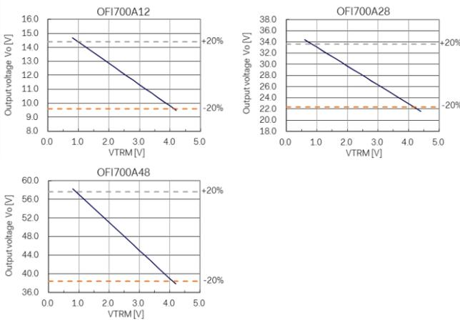
Fig. 4.1 Output voltage by external voltage source
