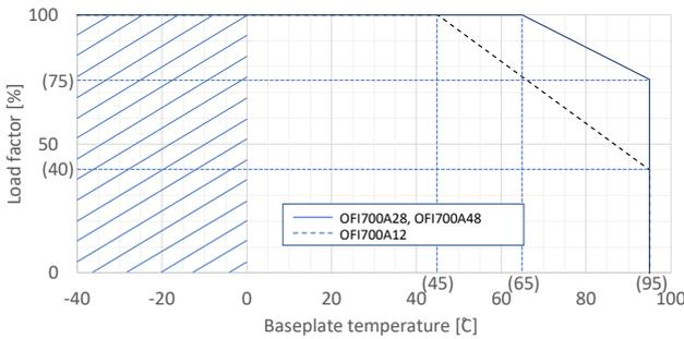
Fig. 2.3 Derating curve of point A (baseplate temperature)
