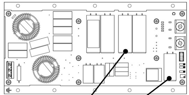
Fig. 6.1 Temperature measuring point for Life expectancy
