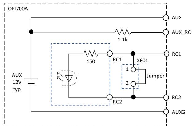
Fig. 4.3 Internal circuit diagram of Remote ON/OFF
