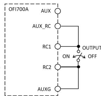
Fig. 4.4 Example of connecting remote ON/OFF circuit
