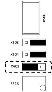
Fig. 4.2 X601 Jumper position
