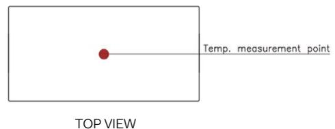
Thermal test condition with vertical direction by natural convection (20LFM).
