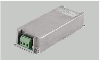
165 x 61 x 35mm very low profile Industrial or ruggedized for harsh environment Many output configurations available Conduction cooled 100°C baseplate
