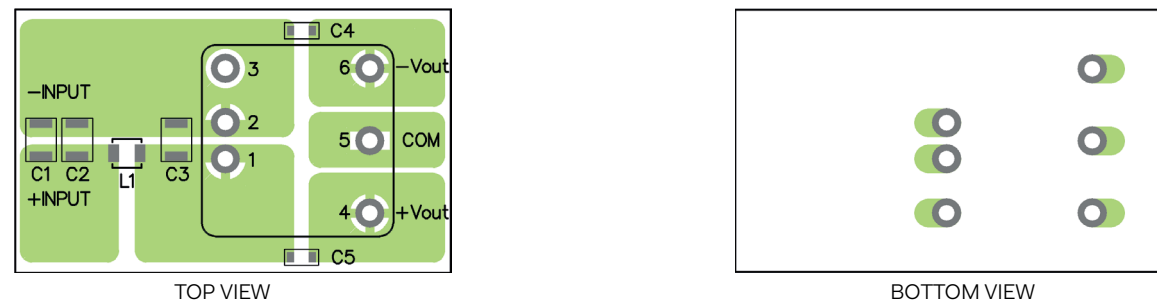
Fig. 4-6 Recommended layout pattern for Dual Output
