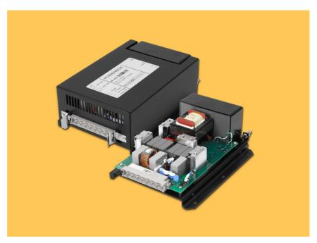
The precharger converts the battery nominal bus voltage of 50VDC up to 137.5VDC to a regulated output voltage of 400VDC or 600VDC to charge high voltage capacitor banks used to switch electric valves actuators such as for unlocking and lifting pantographs
