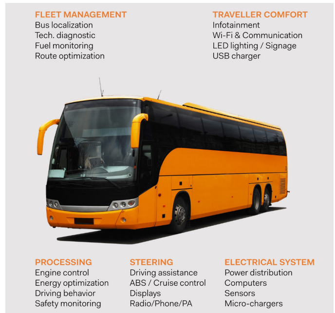
Figure 3 – Applications installed in modern buses, requiring stable power and some local battery for safety operation.
