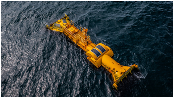
Figure 05: Mocean Energy Blue X Wave Energy Converter (WEC) - (Picture credits: With courtesy of Mocean Energy - Colin Keldie - EMEC)
