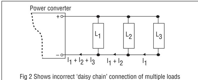
Fig 2 Shows incorrect 'daisy chain' connection of multiple loads
