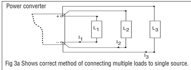
Fig 3a Shows correct method of connecting multiple loads to single source.
