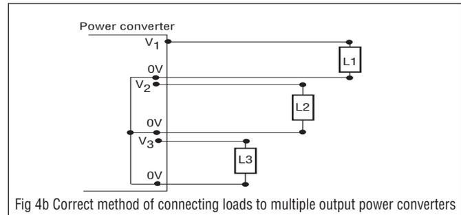
Fig 4b Correct method of connecting loads to multiple output power converters
