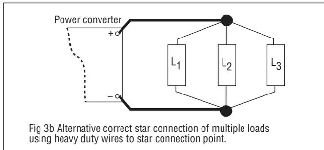
Fig 3b Alternative correct star connection of multiple loads using heavy duty wires to star connection point.
