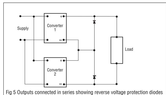
Fig 5 Outputs connected in series showing reverse voltage protection diodes
