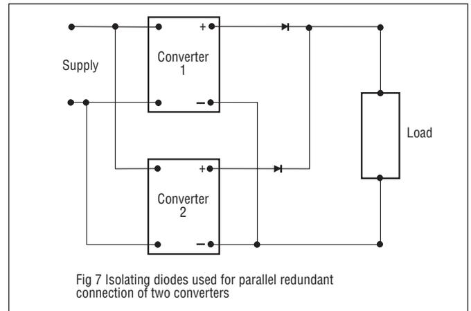
Fig 7 Isolating diodes used for parallel redundant connection of two converters
