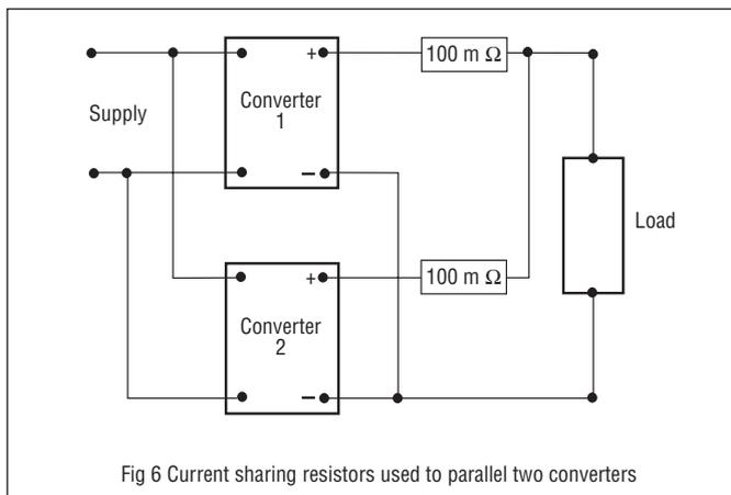
Fig 6 Current sharing resistors used to parallel two converters
