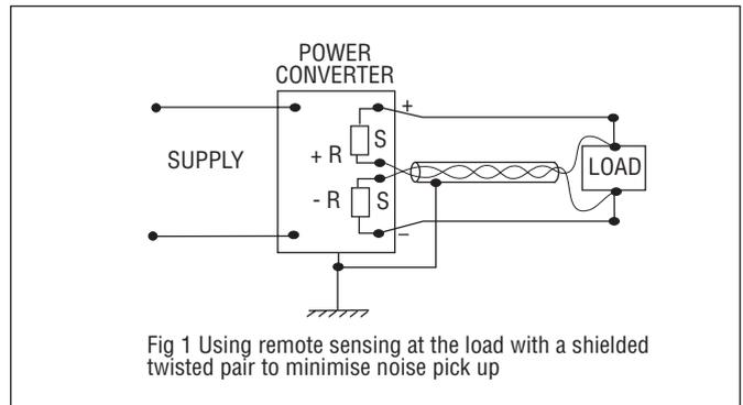
**Fig 1 Using remote sensing at the load with a shielded twisted pair to minimise noise pick up**
