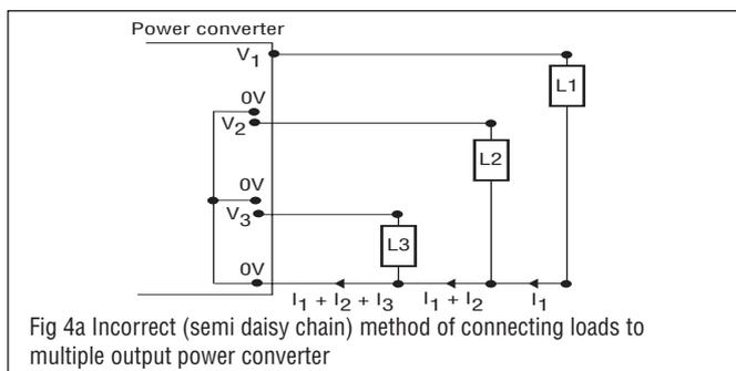
Fig 4a Incorrect (semi daisy chain) method of connecting loads to multiple output power converter
