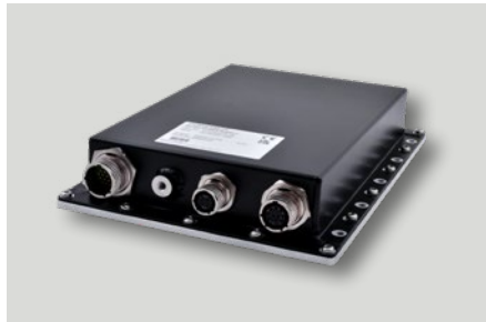
Defense line ECDD DC 250W & 350W, sealed IP65, rugged design DC/DC converter, baseplate cooled, 11- 33VDC or 18-33VDC input, MIL-STD-1275, 461, 810 compliant
